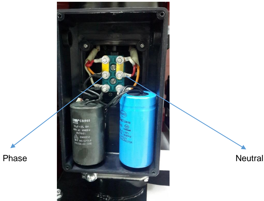
Photo 5. Connection on 220 V AC mono phase motors*
