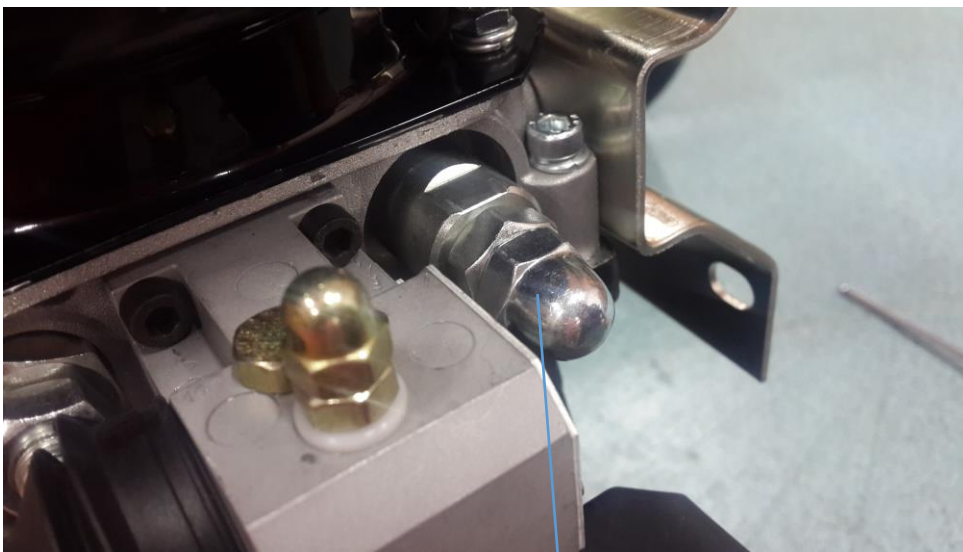
Photo 9. Pressure relief valve
