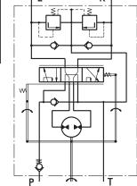
incorporates an axially displaced tracing valve and a metering pump in one housing. The working liquid is supplied by a separate pump and then is directed by the metering pump to the steering cylinders.
