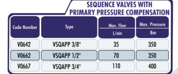
Note: Standard pressure setting range is 30-180 bar. (Set to 90 bar.) Please contact us for other options. For 3/4" standard pressure setting range is 50-400 bar. (Set to 180 bar.) Please contact us for other options.
